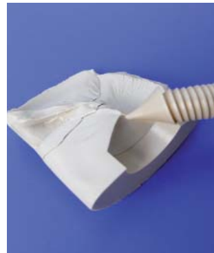
Rupture due to large chip removal
